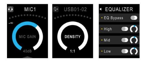
The auto gain compressor has an ON/OFF button and one wheel to set its density.
