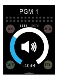
ON: At least one channel is turned on and the fader is opened MIC: At least one microphone one is turned on and is opened
