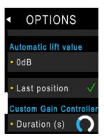
**0dB:** The fader moves to 0dB when opened, to -infinite when closed (default on previous firmwares) **Last position:** Returns to the last position where the finger was lifted off fader (**new** default).
