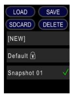
Select the snapshot from the list and press the LOAD button. The current channel / mixer settings are overwritten by the loaded snapshot.
