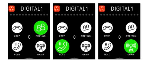
According to the configuration of b-line you can do preliminary talks (PRETALK), put the caller in waiting position (HOLD) or assign hin to one of the channels (ONAIR).
