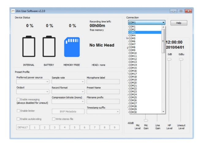
The upper screenshot displays that COM3 has been assigned for communication with iXm. You will need to set the appropriate COM port in *User* or *Admin Software* (see *User Software* below).
